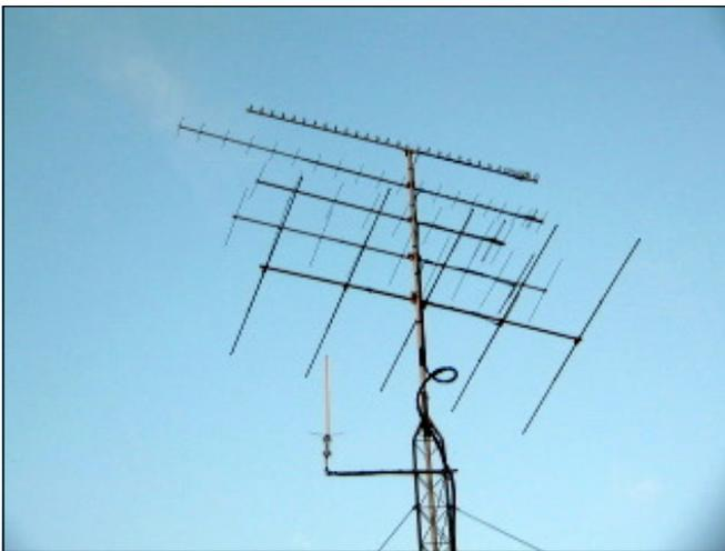
View of top of tower with all antennas- 903, 432, 220, 144 & 6 meter. On side mount is diamond 2/440.
