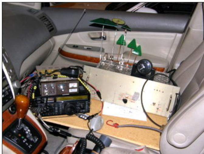
And thanks to **Rick K1DS** for assembling the antennas. I used a 2-position coax switch to route the 2-Meter signal to an antenna, or to the xvtr IF input/output. So all I had to do for microwave use was throw the coax switch, and select desired band on front panel. **A really neat job, Randy.**
